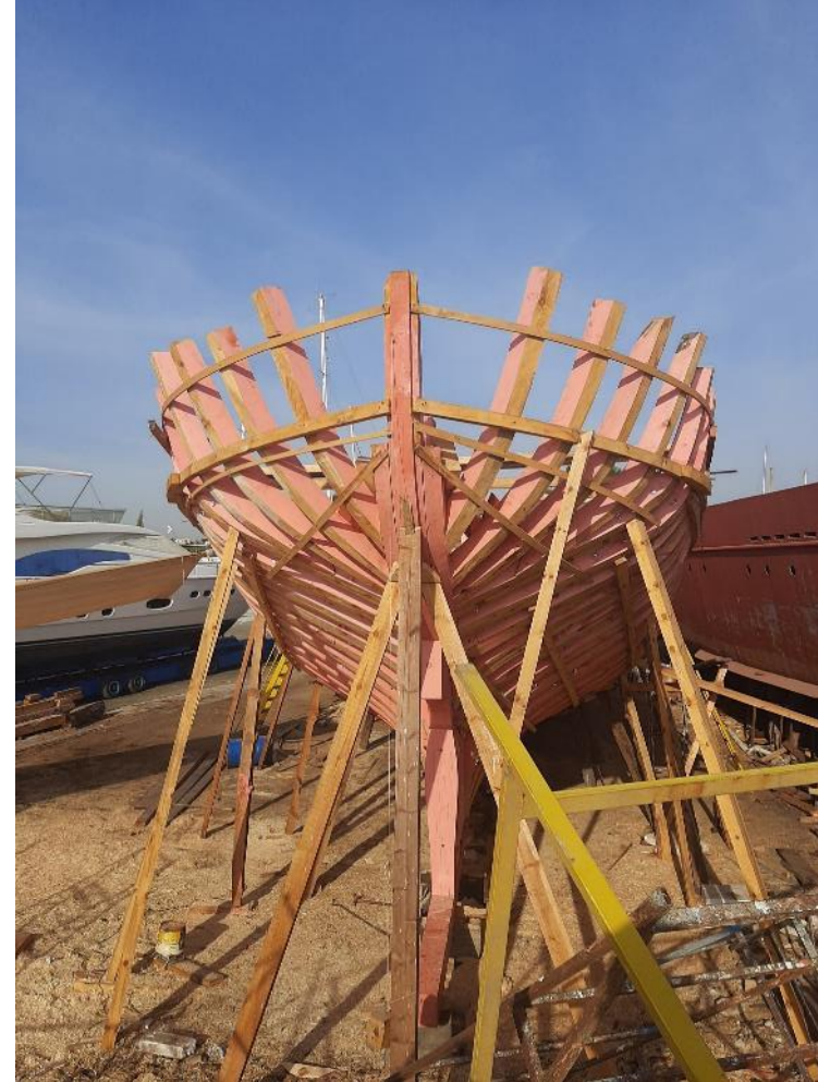
Reconstructed Stern (Back Elevation)
