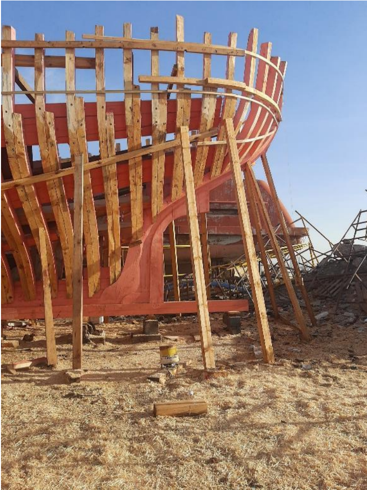
Reconstructed Stern (Side Elevation)
