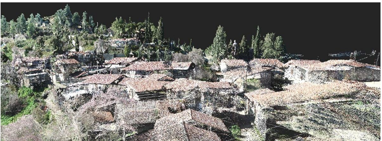
Fig. 9 A 3D point cloud mesh created from drone photography of the village.
