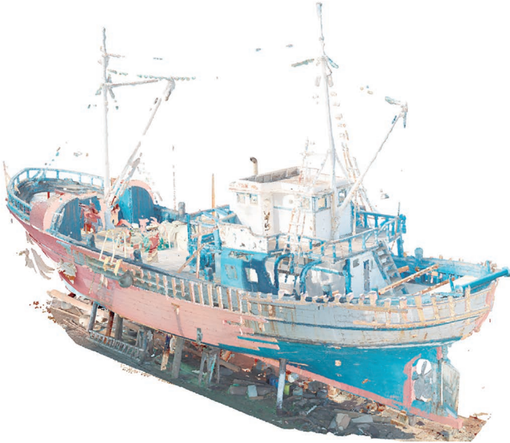
Figure 25. Aligned TLS and Photogrammetric point clouds
