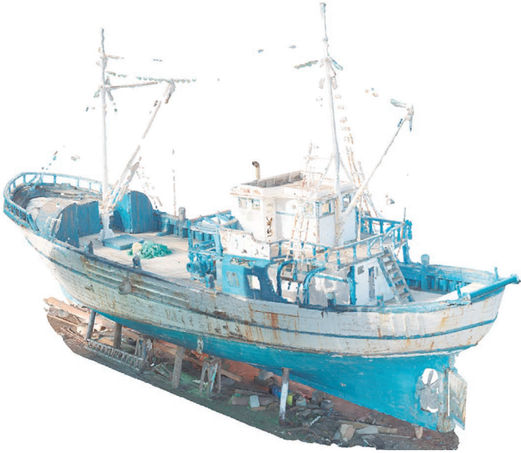
Figure 24. UAV Photogrammetric Point Cloud
