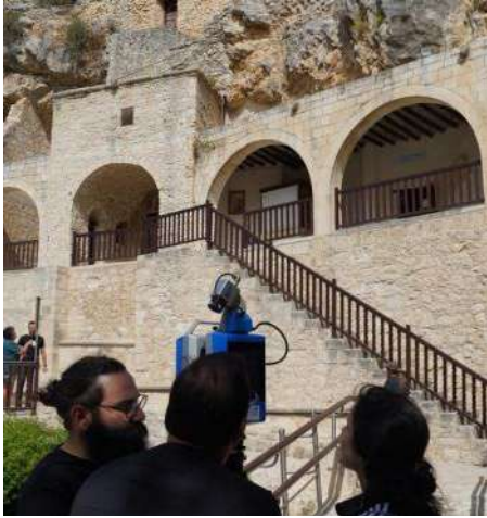
Digitising the Enkleistra using a terrestrial laser scanner
